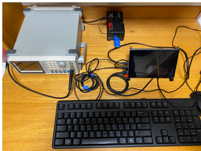
Figure 1. Experimental Setup. A Raspberry Pi 4, along with a monitor and its charging and connection cords, was used to interface with the MPU6050 (not shown) to record frequency and amplitude values of tremors. The PASCO String Vibrator, powered by the Instek AFG-2125 function generator, was used to input frequencies for trial testing.
