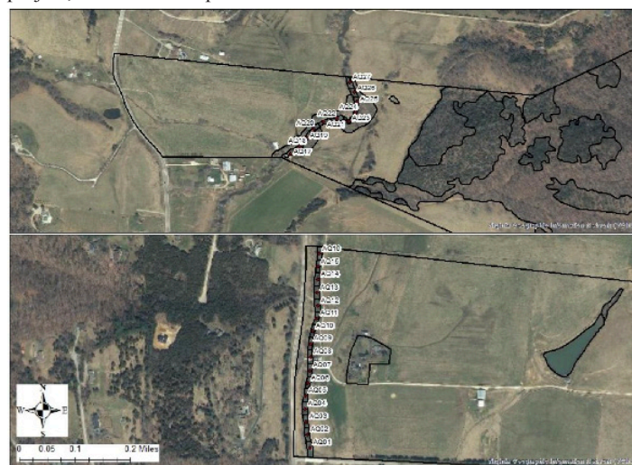
Figure 2. Sample reach distribution in the North (top map layer) and South (bottom map layer) parcels of the North Fork Roanoke River flowing through the study site. The North parcel is upstream of the South parcel. The North parcel river channel is far more sinuous than the South parcel. Sample reaches were 30 m long with 16 reaches in the South and 11 reaches in the North parcel due to the differing lengths of the parcels.
