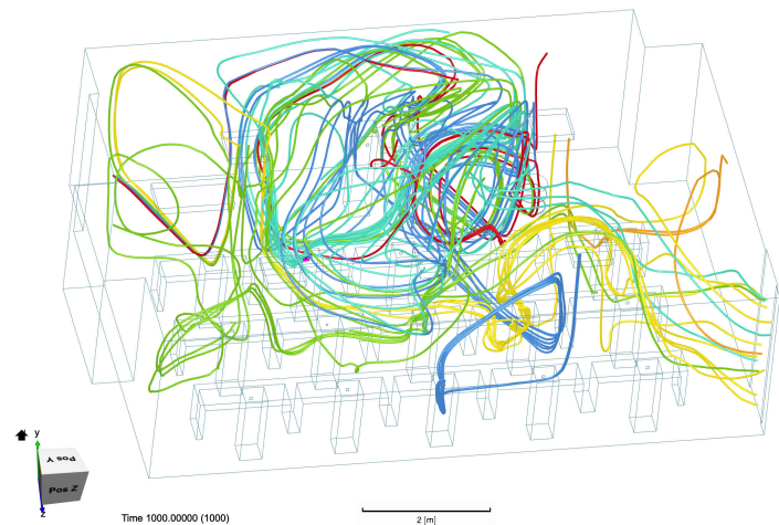
Figure 26. The first of two angles of the same set of particle tracers. Each tracer color represents the exhalation from a different student. Not all students' exhalation paths are shown. A large vortex forms in the middle of the room with a mix of many different colored tracers. Other regions of the room receive less circulation.
