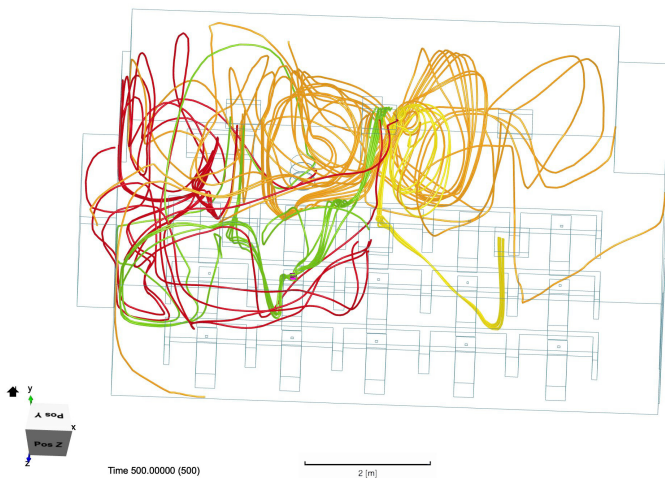
Figure 28. The first of two scenarios where the same circular AP is placed in two different locations. Each tracer color represents the exhalation from a different student. Not all students' exhalation paths are shown. In both scenarios, the exhalation flow becomes jumbled near the AP and does not cycle throughout the room. In Figure 28, several spirally vortices can be seen in the region adjacent to the AP highlighted by orange and red tracers. In Figure 29, a mix of yellow, green, red, and blue tracers concentrate near the AP.
