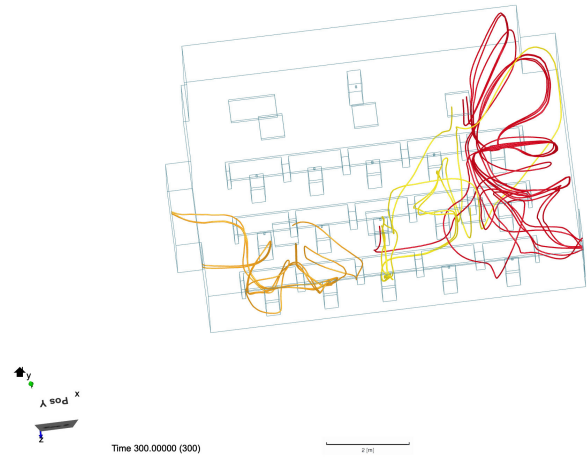
Figure 15. The first of two angles of the same set of particle tracers. Each tracer color represents the exhalation from a different student. Not all students' exhalation paths are shown. With the window and door open, we see air escaping both the right and left sides of the room. The concentration of exhalation noticeably decreases on the left side of the room compared to Figures 11 and 12.
