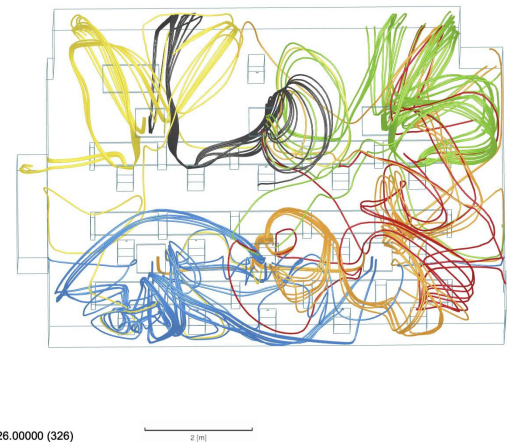
Figure 11. The first of two angles of the same set of particle tracers. Each tracer color represents the exhalation from a different student. Not all students' exhalation paths are shown. The exhalation naturally forms vortices that cycle in various corners of the room as depicted by the different tracer colors. Pockets of heavy cross contamination form as a result.
