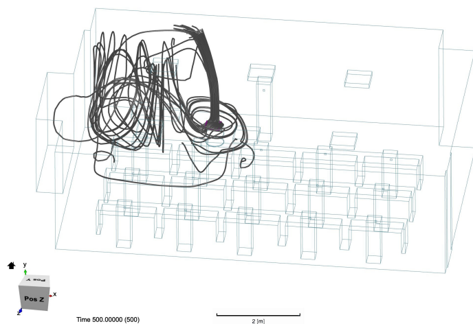
Figure 7. The dark grey particle tracer lines depict the flow pattern of the filtered air after it exits the AP. We see that the clean air ejects from the top of the AP and flows more sporadically throughout the room, concentrating in the region adjacent to the left of the AP.
