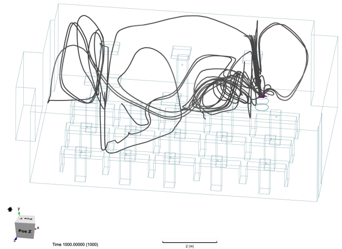
Figure 25. The dark gray particle tracer lines depict the flow pattern of the filtered air after it exits the AP. We see that the clean air ejects from the top of the AP and flows more sporadically throughout the room, concentrating in the region adjacent to the left of the AP. The same AP from Figure 7 is moved to another location. The clean air flow patterns follows that of Figure 7, where clean air concentrates adjacent to the AP and does not circulate throughout the room.
