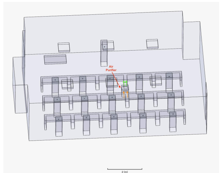
Figure 5. The arrangement is the same as that of the full room described in Figure 1 and the box-shaped AP is the same as described in Figure 3. However, the AP is now moved to the middle of the room in between students' desks and turned to align with the z-axis.
