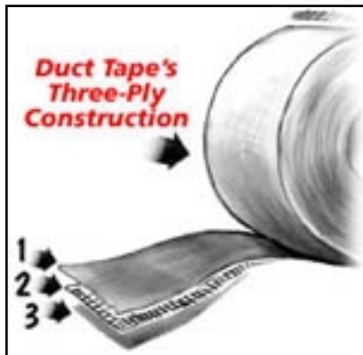
Figure 2. Duct tape is composed of three layers. A layer of fabric mesh (2) is enveloped by a layer of rubber-based adhesive (1) and a layer of polyethylene plastic (3). Courtesy of Duct Tape Guys .
